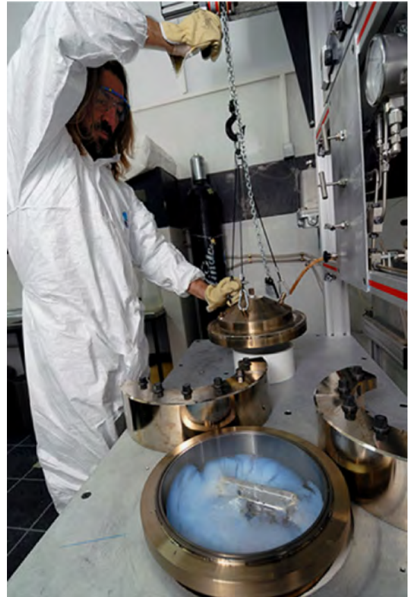
Fig. 3. Supercritical drying apparatus. The artist opening the vessel after 48 h of constant running. Photograph and ©Massimo Pizzocaro, 2008.
