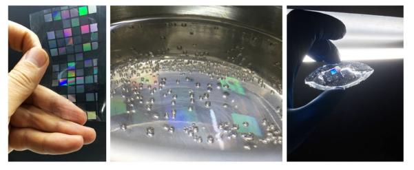
Fig. 10 (Left) The PET film with the rainbow hologram motif to be transferred onto the alcogel. (Middle) The PET is placed onto the mold and alcogel is poured into the mold; bubbles are trapped because of a very fast gelation. (Right) The rainbow hologram motif is extremely
